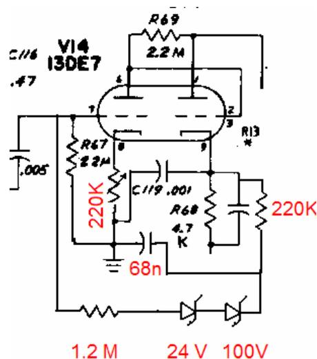
Controlled Carrier AM Modulator with ALC
